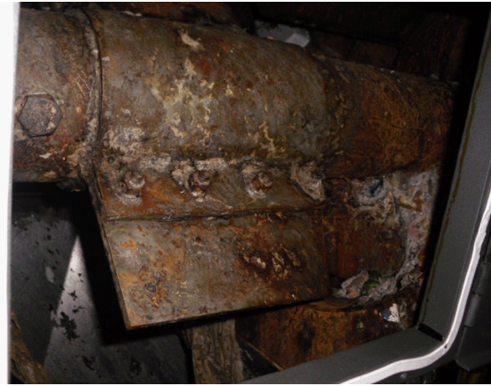
Counter spire and/or thrower plate (flat to ensure the product comes out)
